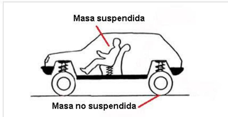
**Figura 2-2:** Masa suspendida y no suspendida
