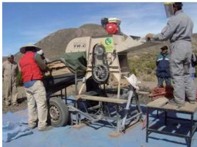
**Figura 7-2:** Trilladora TR-C
