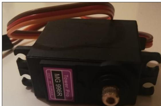
**Figura 18-2:** Servo motor MG996R
