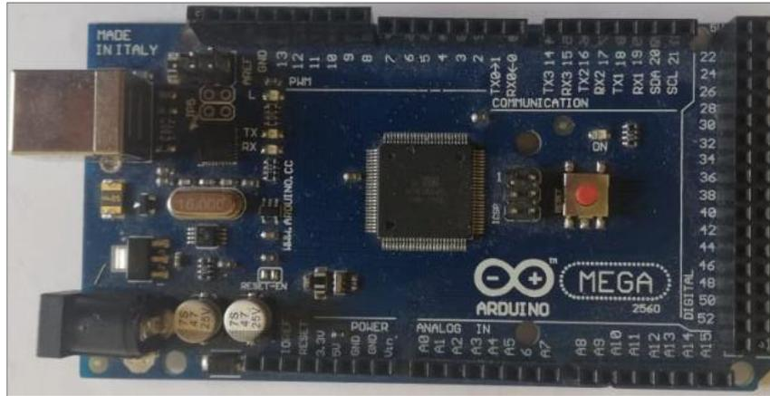
**Figura 9-2: Arduino Mega2560**
