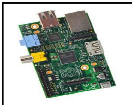
**Figura 5-1:**Tarjeta Raspberry Pi.
