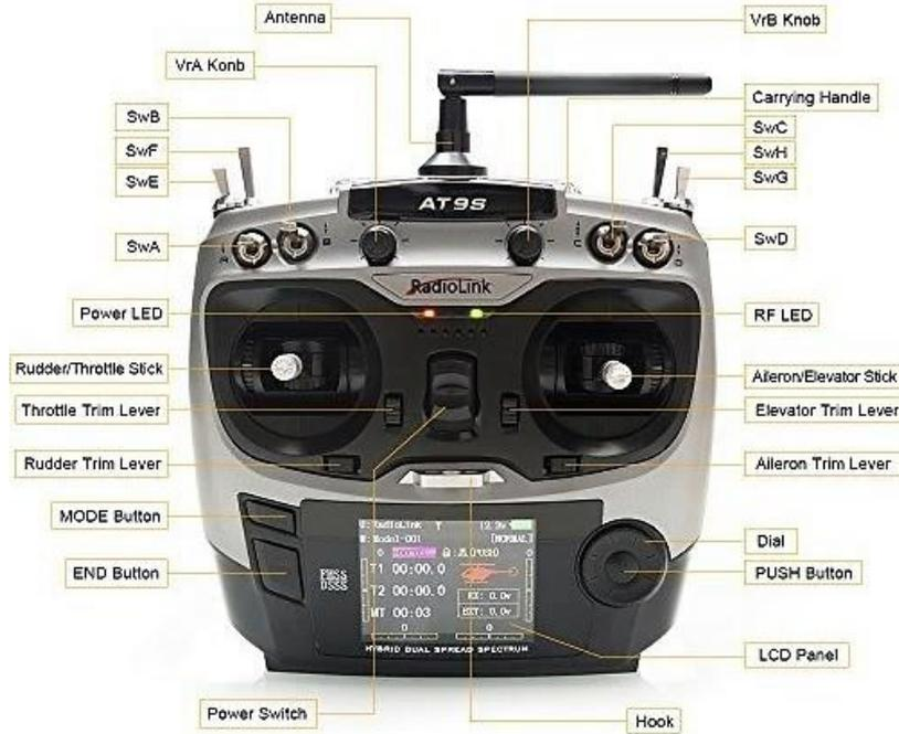
**Figura 25-2:** Componentes del radio control RadioLink AT9S
