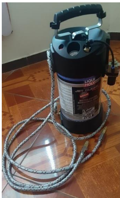
Figura 7-2: Tanque Canister Liqui Moly
