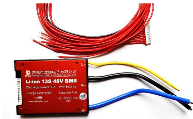
Figura 28-3: BMS DALY 13S 48V 30A, separate port
