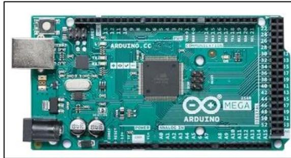
**Figura 6-3:** Arduino Mega 2560
