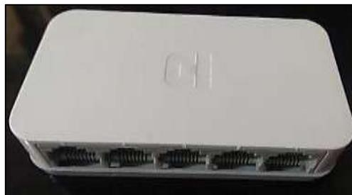
**Figura 15-3.** Switch D-Link DS-1005A
