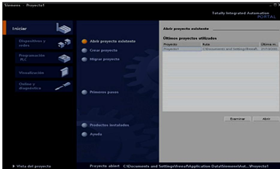
Figura IV-5: Vista principal del TIA Portal del software STEP 7
