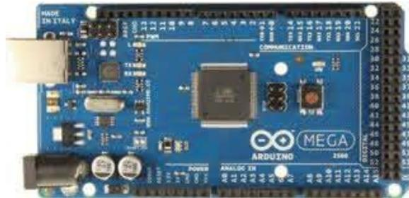
**Figura 8-2.** Arduino MEGA.
