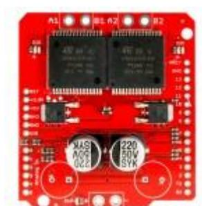
**Figura 11-2.** Motor Shield VNH2SP30.
