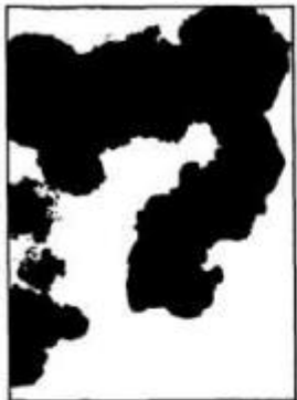
Rust Grade 2-S, 33% Rusted
