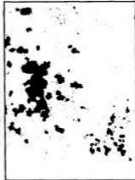
Rust Grade 4-G, 10% Rusted
