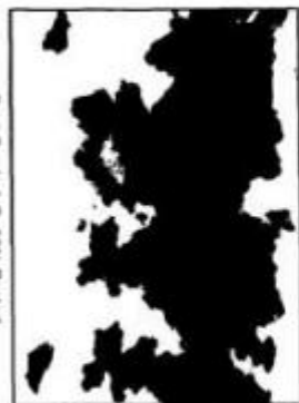
Rust Grade 2-G, 33% Rusted
