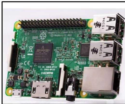
**Figura 2-3.** Raspberry Pi Modelo 3B
