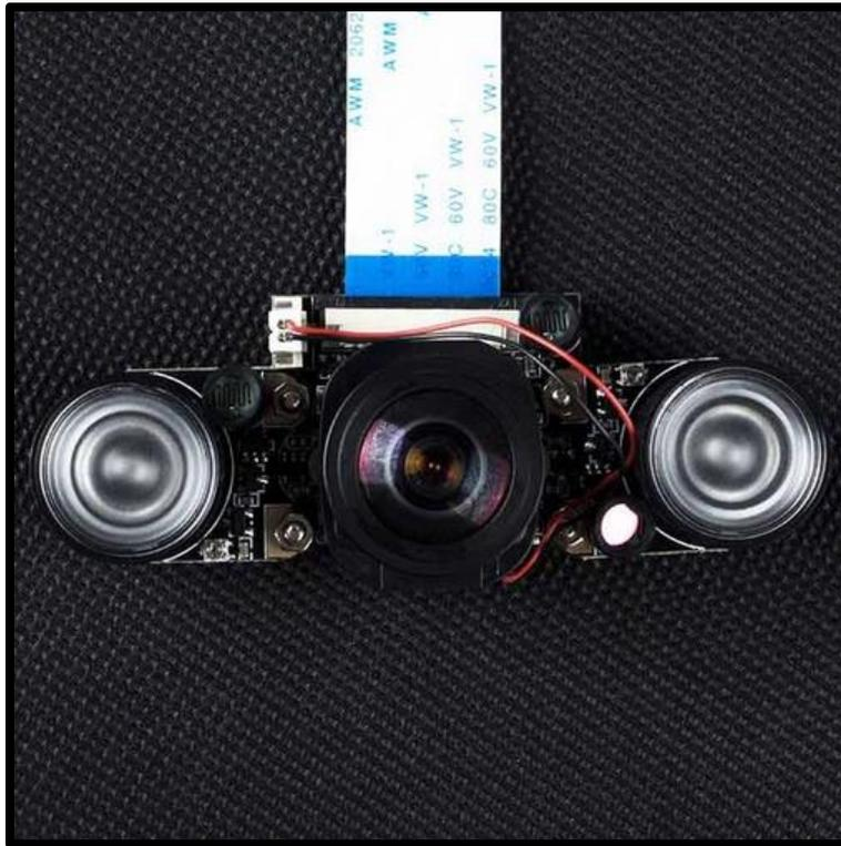
**Figura 11-1.** Raspberry Pi Camera Board
