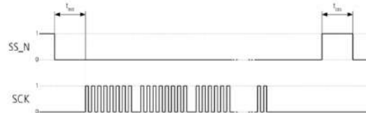
Figure 3: SPI timing diagram
