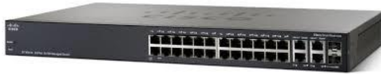
Figura 2-3: Switch cisco SF 300 de 24 puertos
