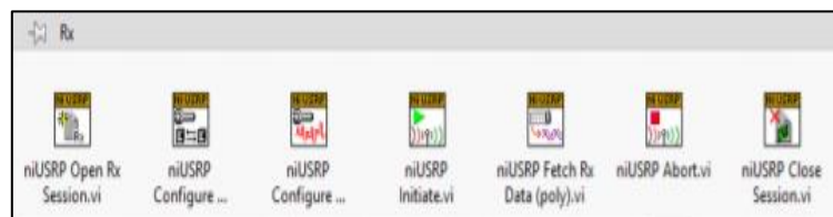
Figura 33-3: Bloques RX USPR de LabView.
