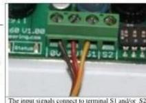
The input signals connect to terminal S1 and/or S2
