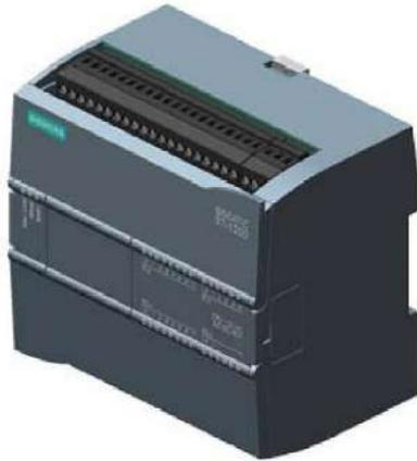
SIMATIC S7-1200, CPU 1214C, CPU COMPACTA, AC/DC/RELES, E/S INTEGRADAS: 14 DI 24VDC; 10 DO RELES 2A; 2 AI 0 - 10V DC, ALIMENTACION: AC 85 - 264 V AC BEI 47 -63 HZ, MEMORIA DE PROGRAMA/DATOS 75 KB
