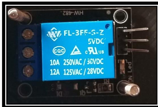
**Figura 4-3:** Relé Arduino 5VDC.
