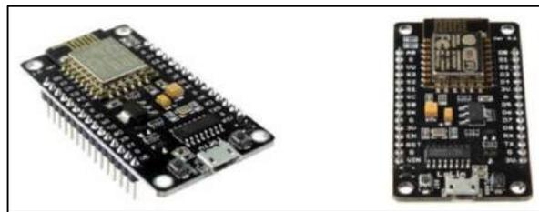
Figura 5-2: NodeMCU ESP8266
