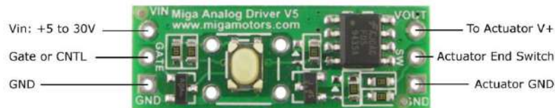
Miga Analog Driver V5 -Pinout Diagram
