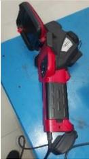
A red and black handheld infrared camera with a lens and a viewfinder, used for non-destructive testing.               |
