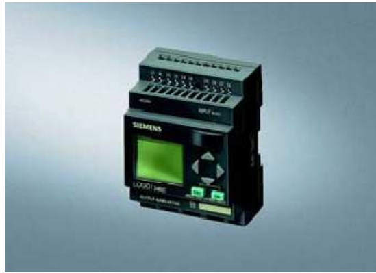
Figura II- 11. Plc Logo Siemens 12/24 RC
