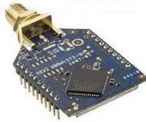
**Figura 3-10** Xbee 900 RPSMA
