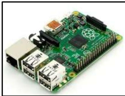
**Figura 22-1** Tarjeta Raspberry Pi.
