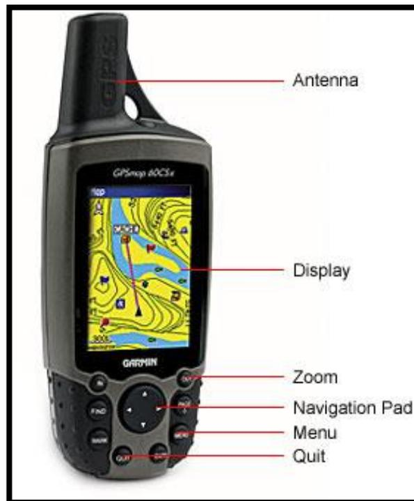
**Figura 2-4** GPS Garmin GPSmap® 60CSx
