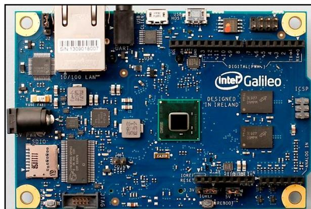
**Figura 1-9** Tarjeta Intel Galileo
