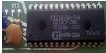
**Figura II.16:** General Instrument PIC1650
