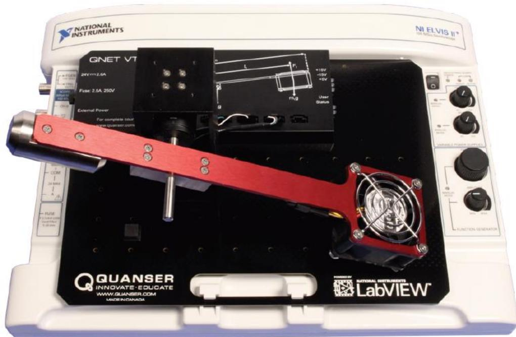
**Figura 1-3:** Quanser QNET 2.0 Vertical Take-Off and Landing Board para el NI ELVIS II.
