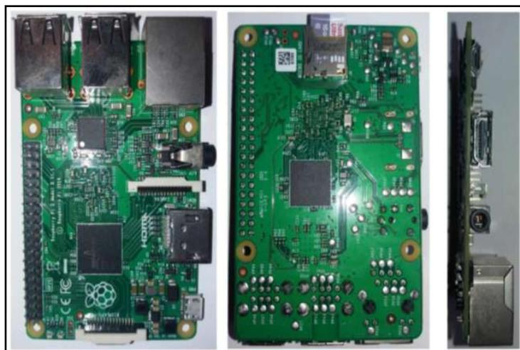
**Figura 8-2:** Raspberry pi 2 modelo B
