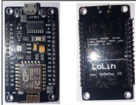
**Figura 9-2:** Placa NodeMCU v2.
