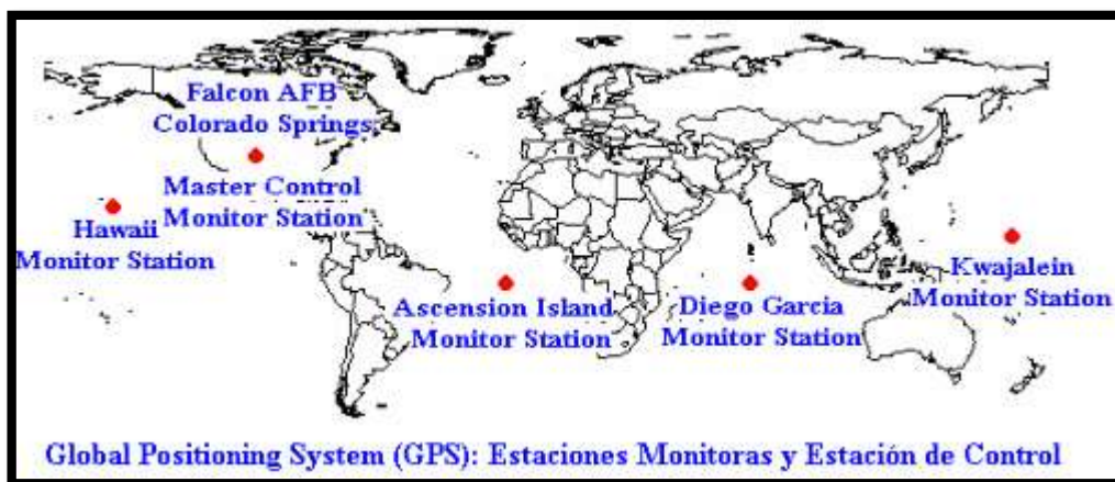
Figura 5-2: Segmento de Control GPS
