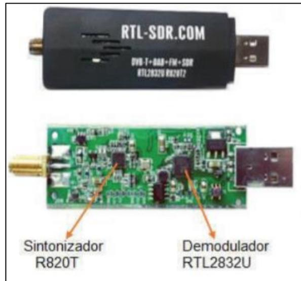
**Figura 8-1** Modulo RTL-SDR
