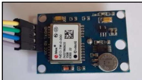
**Figura 7-2:** Módulo GPS Neo-7M
