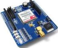
IComSat is a GSM/GPRS shield for Arduino and based on the SIM900 Quad-band GSM/GPRS module. It is controlled via AT commands (GSM 07.07 ,07.05 and SIMCOM enhanced AT Commands), and fully compatible with Arduino / Itarduino and Mega.
