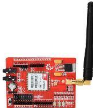
Figura 18-2: Tarjeta SIM900A GSM/GPRS
